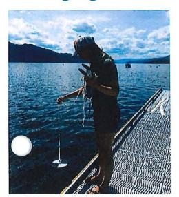
Staff prepare to lower a Secchi disk to take a water quality reading. The Secchi disk gives an indication of water clarity.
